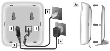
Insert the phone cable into the right-hand connection socket 1 at the rear of the base until it clicks into place.
